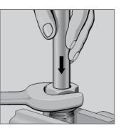
Standard manual assembly using the pre-assembly adapter
