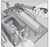
Assembly with the MHH-R manual pre-assembly unit
