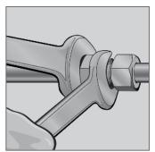
Complete manual assembly in the fitting body
